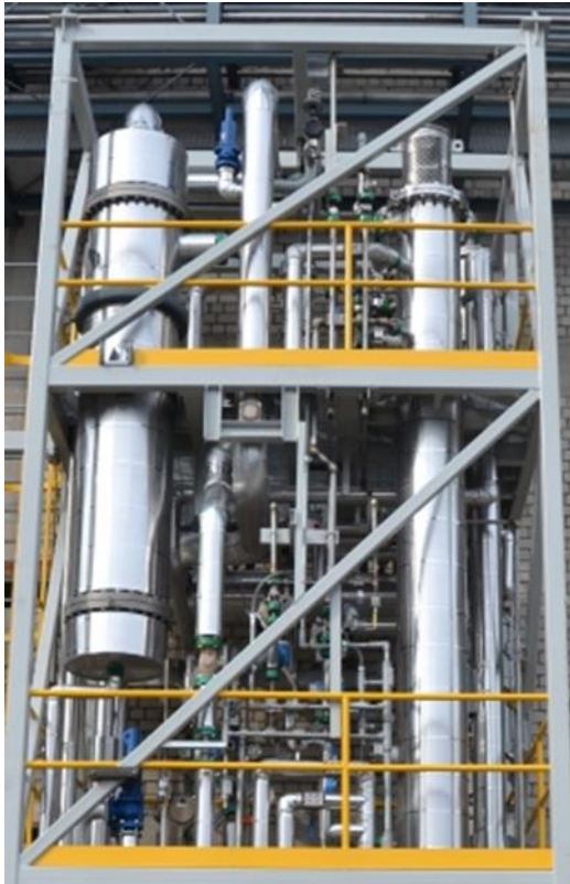
Figure 10: Counter-current extraction by AVA Biochem to extract HMF from the aqueous product solution. (Image: AVA Biochem)
